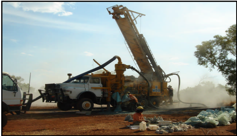
Photograph 1: RC drilling at Flamingo during early November 2009
